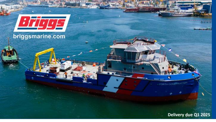
Briggs Marine's versatile Maintenance Support Vessel measures 40 metres in length and boasts DP2 propulsion as well as additional features including a heave compensated crane, a moonpool, a detachable A-frame, a 4-point mooring system, and a survey project office. Additionally, the design incorporates a demountable Crew Transfer Vessel (CTV) boarding ladder to enhance its ability to support offshore windfarm projects.
